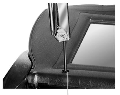
3 Remove the four T-8 torx screws from the corners of the display.
