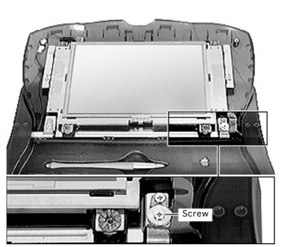
7 At the bottom right corner hinge, use a Phillips #0 jeweler's screwdriver to remove the bottom screw and washer.
