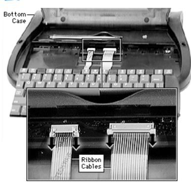
4 **Caution:** Do not use pliers or a screwdriver to remove the ribbon cables: this could damage the traces on the cables.
