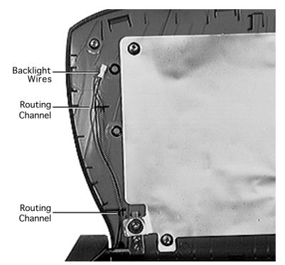
2 Route the backlight connector wires out of the routing channels.
