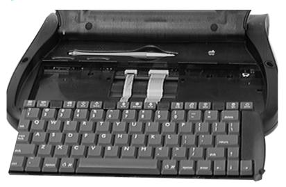
Replacement Note: Before replacing the keyboard, make sure the ribbon cables are securely connected and folded. Tilt the keyboard so the top is secured first, then use a flat-blade jeweler's screwdriver to press the bottom of the keyboard until it snaps into place. (Refer to the graphic in step 1 for the three places to press.)
