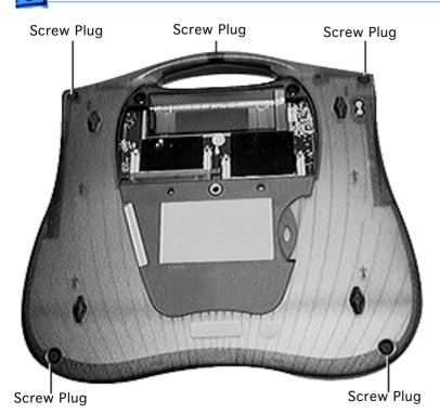
Remove the four round corner screw plugs and the oval handle screw plug from the bottom case.
