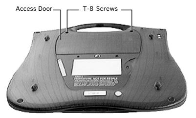
1 With the display lid closed, turn over the eMate and use a T-8 torx driver to remove the two screws from the access door.
