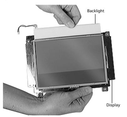
2 Using your fingers or a needlenose pliers, grasp the backlight's clear plastic edge and slide the backlight out of the display assembly.
