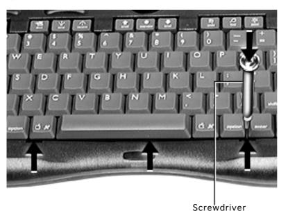
Use a flat-blade jeweler's screwdriver to pry up the keyboard in three places indicated in the graphic.
