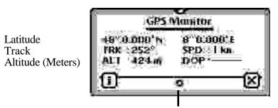
Longitude Speed (kilometers) Position Quality (PDOP) The small flashing symbol below the text field will change each time a GPS update occurs. That should happen at least all five seconds to be compatible with GPS Map or GPS Map Lite.
